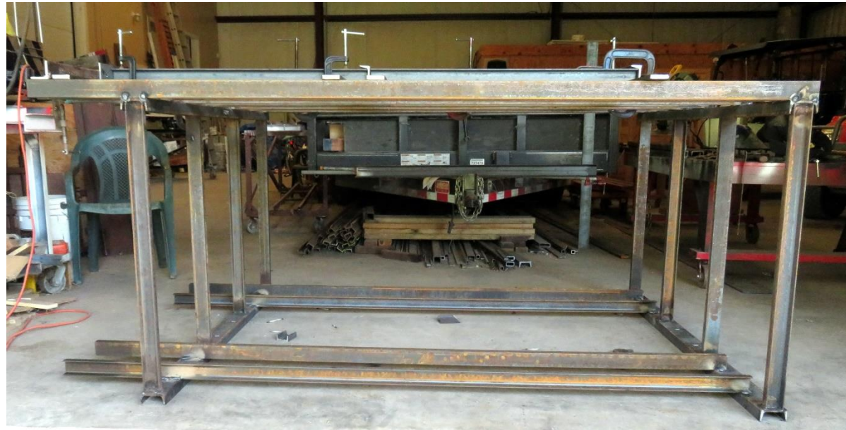
Three track wide rack being used as a jig. Rusty steel is the jig. Black steel is the support being aligned to the jig.
