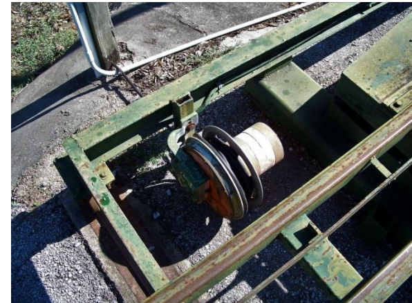
Be careful with the transfer table. The return spring is broken in the cord winder so it ends up laid out and liable to be run over and cut.
