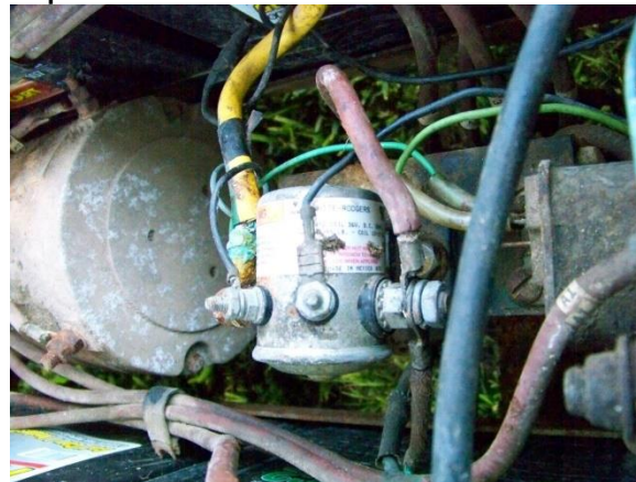
This is the device I had to bypass in order to use speed and reversing controls. Hooked up the yellow to the faded red on the right with a jumper cable.
