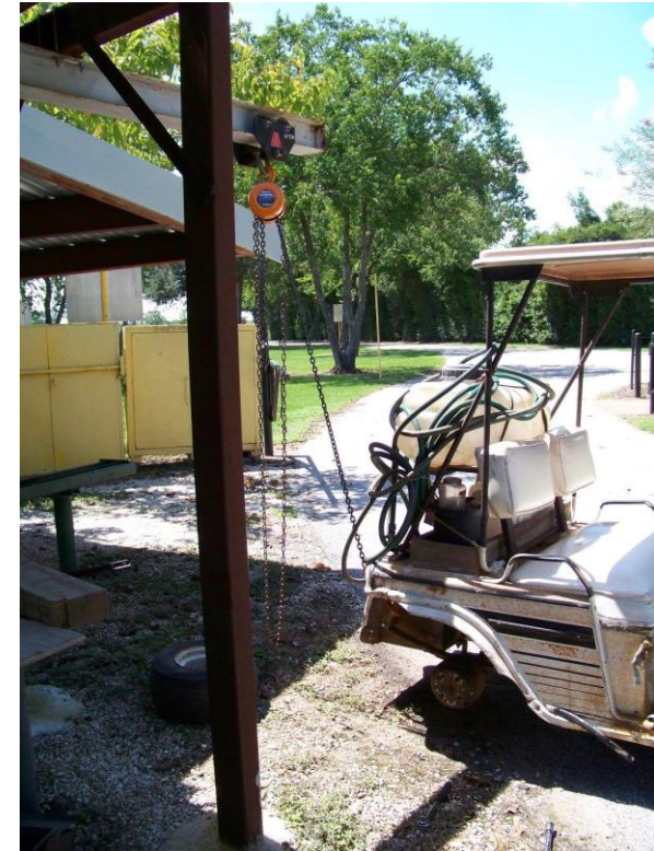
Hoist holding up golf cart.
