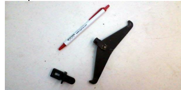
The parts Bill Howe found. Doug Blodgett: It's mine. I checked that rigging just a couple of weeks ago and it was fine. Looks like the turnbuckle just worked itself loose and the crossover link finally dropped off.
