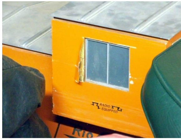
Damaged exterior, revealing plywood underneath.
