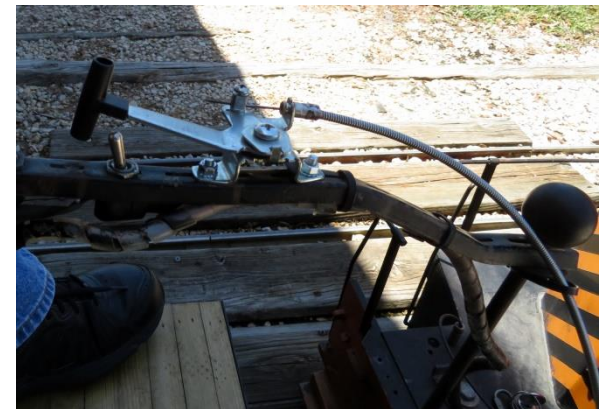
Throttle on HALS 5321 has been moved to where you can reach it. Great addition, thanks Gary.
