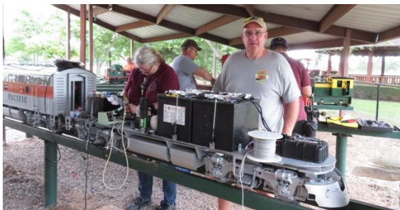
Laura Walter is fixing JB Cason's sound system in his Western Pacific unit. She designed and built the sound units.
