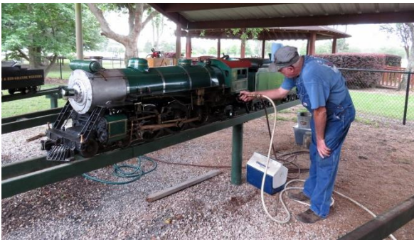
JT Bailey connecting water to his boiler. Friday
