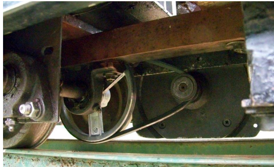
New belt and pulley underneath. Pulleys are a weak link, this one has already been warped in a derailment, but still better than before.
