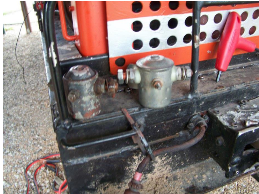
Old beat up solenoid on the left, replacement solenoid on the right may be just as old, but has lived a much easier life so far.
