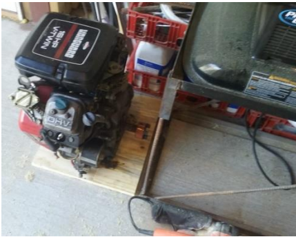
The old gasoline motor has been removed.
