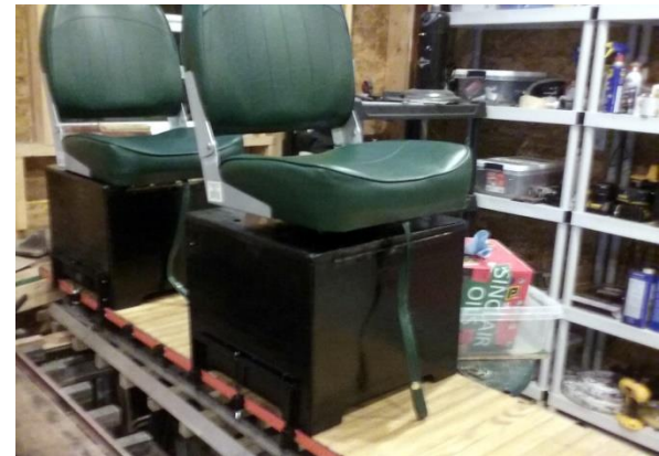
Seats ready for riders. Front seat swivels, back seat fixed position. March 8
