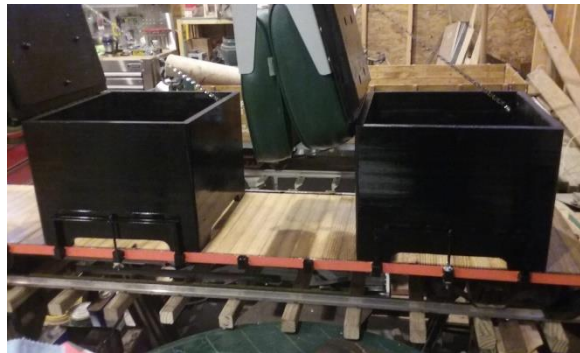
The wood boxes supporting the seats after painting, with hold down and alignments on side of the boxes. Seat boxes open. March 8
