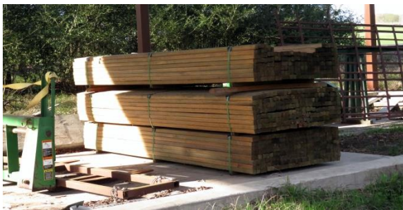
This is all HALS treated lumber for making ties. The HALS tractor "Walt" cannot lift a bundle so I loaded it here where it is under cover, but not inside.
