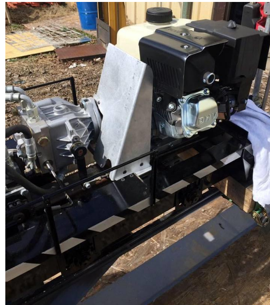
Above: The new heat shield will help keep exhaust heat away from fuel. Cab windows opened more.
