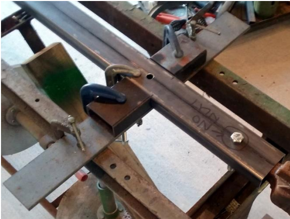
Birth of a new car. First few photos show parts clamped together before welding.
