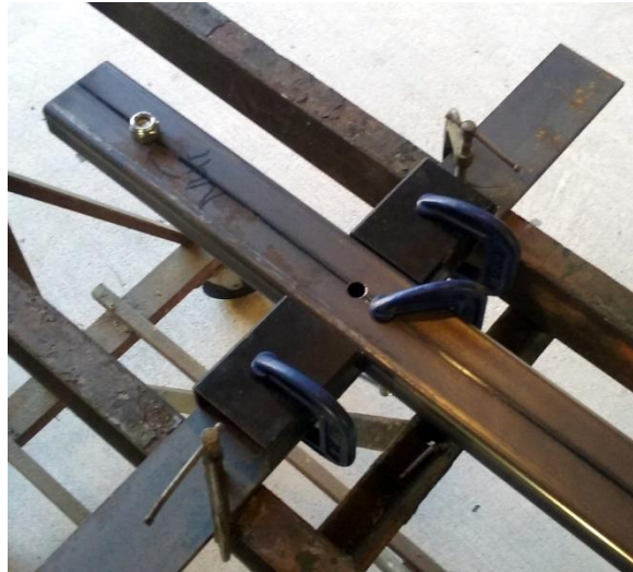
LEFT: Frame in place with 1 x 2 inch coupler pocket sticking out the end. Two plates welded in place with holes for mounting eye hooks for safety chains.
