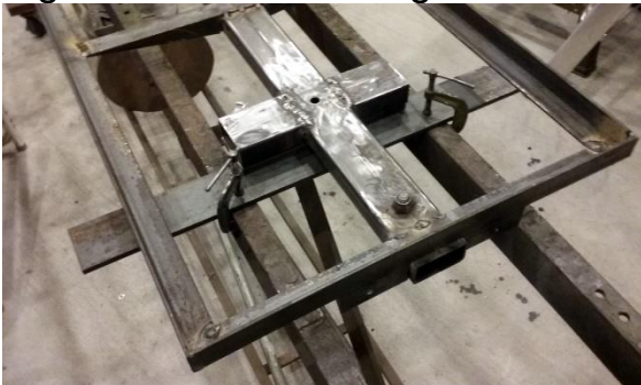
Birth of a new car. First few photos show parts clamped together before welding.
