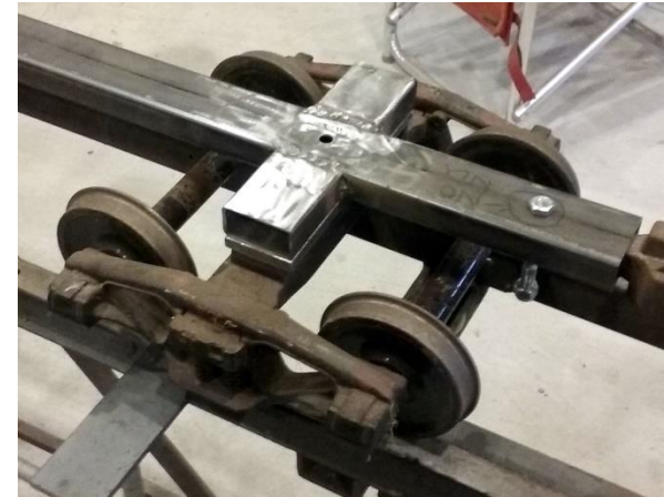
Car's backbone with the cross pieces welded together and the extra plates for Tom Bee trucks bolted on rather than welding it to the frame.
