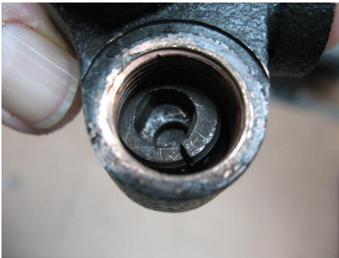
This is the lever arm inside the gate valve. You can see the fracture in the arm where the rectangular hole is. A rectangular rod engages this to swing the gate into place and it was becoming very loose with a lot of slack
