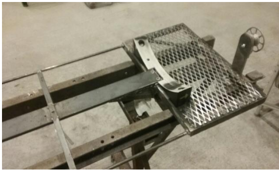
Flat bar 3/8 by 2 inches held in place by screws before cutting main frame.
