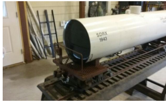
After old main frame cut, just the flat bar under the tank car for strength. Small domes in place. End platforms installed.
