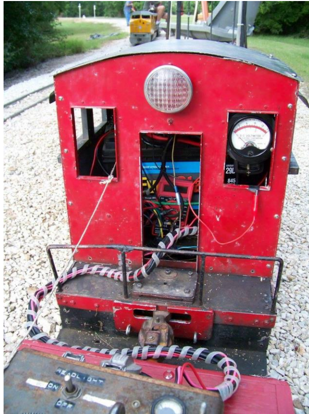
RIGHT: The hard to see (in door way) digital multimeter will be removed eventually. Found a vintage voltmeter that seemed like a good fit. Put it in today, will do some more permanent wiring later.
