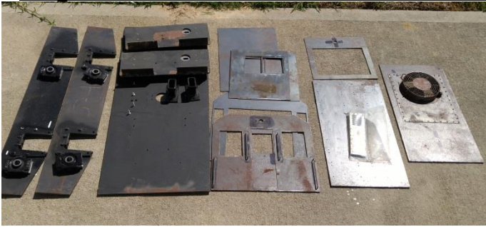
Art Morris critter kit: main frame parts on the left and cab/hood parts on right.
