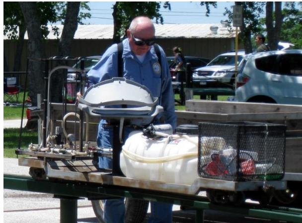
Bill Howe Version 2 of the HALS spray car. Longer, with storage at one end. 2012-0421
