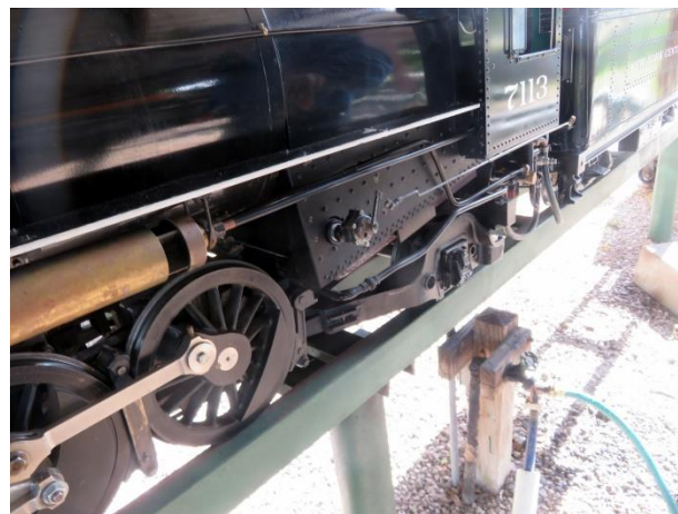
The blow down valve shows on the outside of the fire box behind driver #4.
