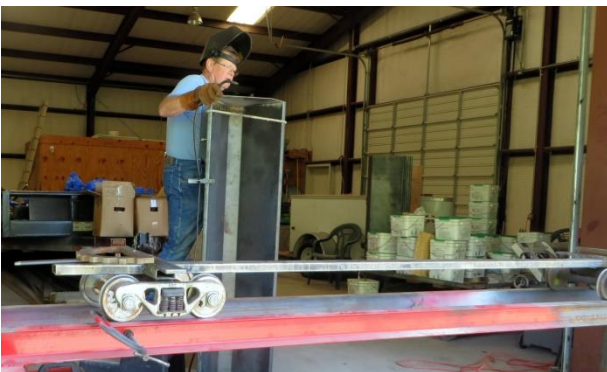
Ed Rains checking his welds. We used a rope to hold the body tight to the end piece. Frame with trucks mounted,, ready for the body. We designed the weight to transfer straight down to the truck bolster and not through any frame pieces. 2014-0410
