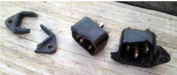
The two replaced sockets. On left from control box, on right from the side of the locomotive where the charge cable plugs in.
