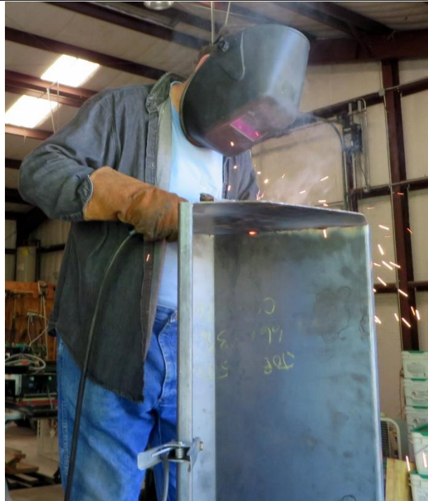
Ed Rains welding on the end of the first car, a trial before doing the other five. Red glow should be there. 2014-0410
