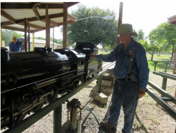
Doug Blodgett working on his blow down valve, it lets the boiler pressure out.
