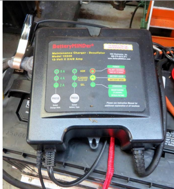
RIGHT: the 12 volt battery charger that Clyde Brown uses. Clyde has this because it fixes sulfated batteries.
